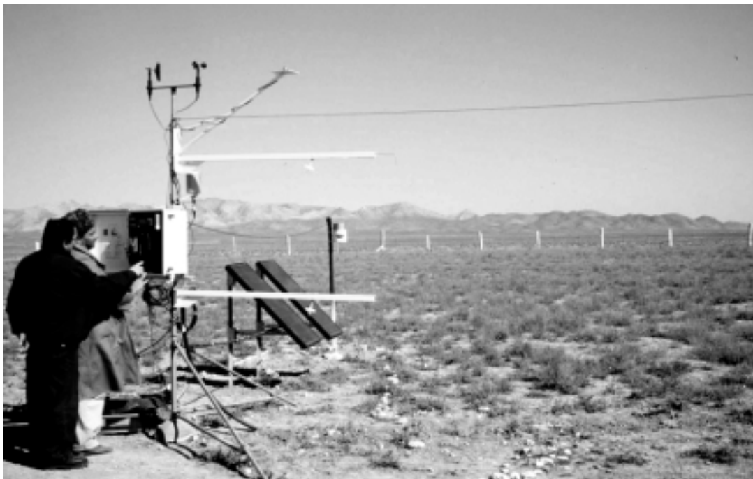
On-site training with the installation of the CO 2 /Bowen ratio-energy balance technique at the CO 2 flux monitoring site (shrub-ephemeroïd semidesert ecosystem) in Karnap, Uzbekistan. K. Akshalov (left) and M. Nasyrov (right)
